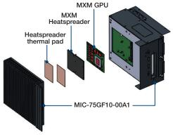
Note 1: Need to order MIC-75GF10-00A1, MXM GPU and MXM heatspreder.
